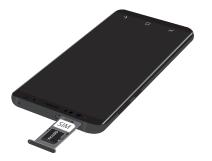
6. Slide the SIM card/Memory card tray back into the slot.
